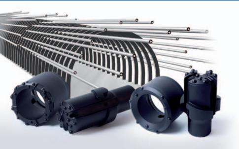
Forepoling, also known as tube umbrella, is an application used to strengthen the tunnel roof in broken rock conditions. The drilling system consists of casing tubes which are drilled through the overburden as an umbrella and filled with grouting. The Robit<sup>®</sup> Casing System allows easy driving of the casing tubes into the ground with low torque demand.
