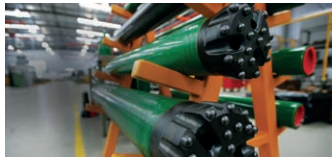
The company's production portfolio includes DTH hammers and bits for the mining industry.
