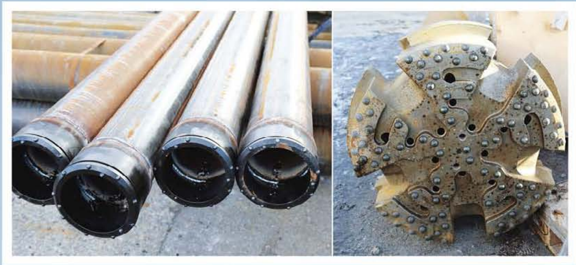
Casings with ring bits and a flow control pilot ready for action at Bjørvika.
