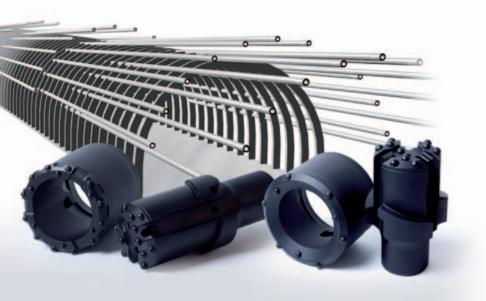
Forepoling, also known as tube umbrella, is an application used to strengthen the tunnel roof in broken rock conditions. The drilling system consists of casing tubes which are drilled through the overburden as an umbrella and filled with grouting. The Robit<sup>®</sup> Casing System allows easy driving of the casing tubes into the ground with low torque demand.
