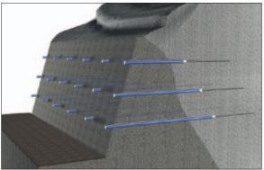
Anchoring is a method by which walls with masses of overburden are anchored to the solid rock. Casing tubes are driven through the overburden. Drilling then continues with a normal drill bit. Steel cable is inserted to the bottom of the hole and the hole is then filled with grouting.
