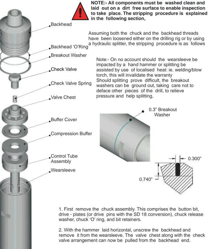
The remaining buffer cover, compression buffer and control tube assembly can be removed by lifting the chuck end of the wearsleeve which will allow the piston to push the parts up to the end face, from where they can be removed by hand.
