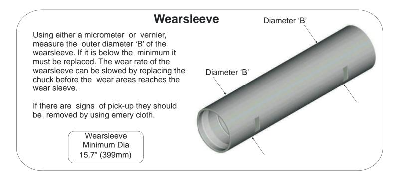
If a piston has broken within the wearsleeve it is imperative that the bore is honed to remove any burrs or 'pick-up'
