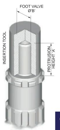
The Robit Hyper 181 hammer is designed to be used with Foot Valves that are to the following specifications:
