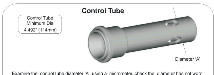
Examine the control tube diameter 'A', using a micrometer, check the diameter has not worn under the specified minimum.
