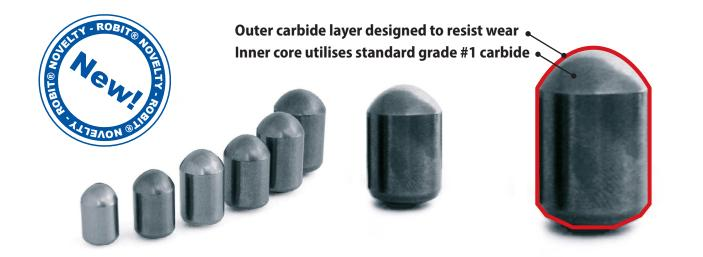
The new **Dual Property Extreme Carbide** has an outer carbide layer that is designed to resist wear, the inner core utilises Robit standard grade #1 carbide. Even when the outer layer has been worn away, the DTH bit performs in the same way expected from the Robit standard quality carbide. The carbide allows for extreme wear resistance but also has a core that is durable to resist fracturing.
