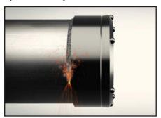
1. Weld the ring bit assembly to the casing.
