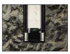
2. Continue drilling the casing until the bedrock and some feets in it.
