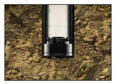
1. Drill the casing through the overburden soil.
