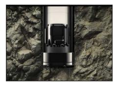
3. Unlock the pilot bit from the ring bit assembly and lift the drill string up.
